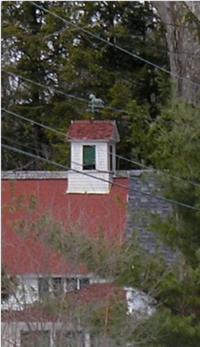
Unusual side gabled roof with Greek revival pediment (matches the side gabled carriage house roof), single rectangle shutters, clapboard sided base, mid-section and gables with mill work complimenting the carriage house's. Northern Maine 19th century.
